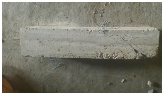
Figure 11: Cracks in Beam no. 2 after Testing
