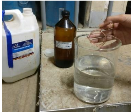
Figure 2: Preparation of Solution for Accelerated Corrosion
