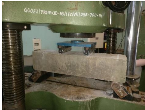
Figure 6: Set Up for Flexure Test
