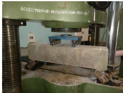
Figure 6: Set Up for Flexure Test
