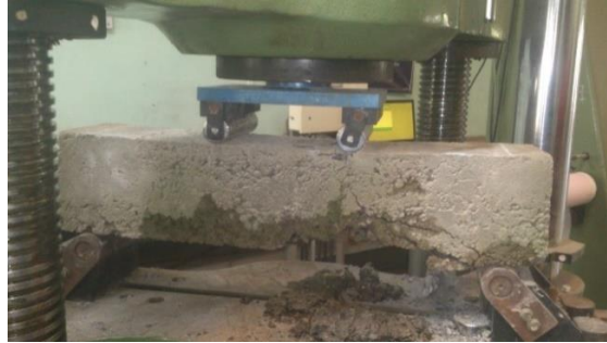
Figure 12: Cracks in Beam no. 10 after Testing
