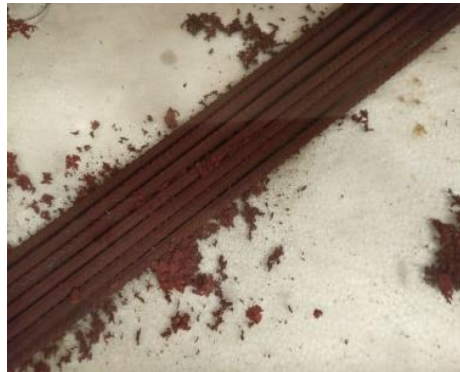
Figure 3: Bars Corroded in Solution
