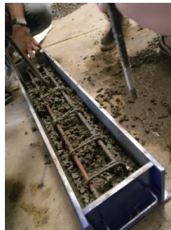
Figure 5: Casting of Beams
